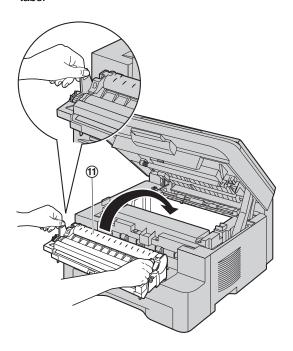
Make sure that the triangles (②) match, to install the drum and toner unit correctly.
